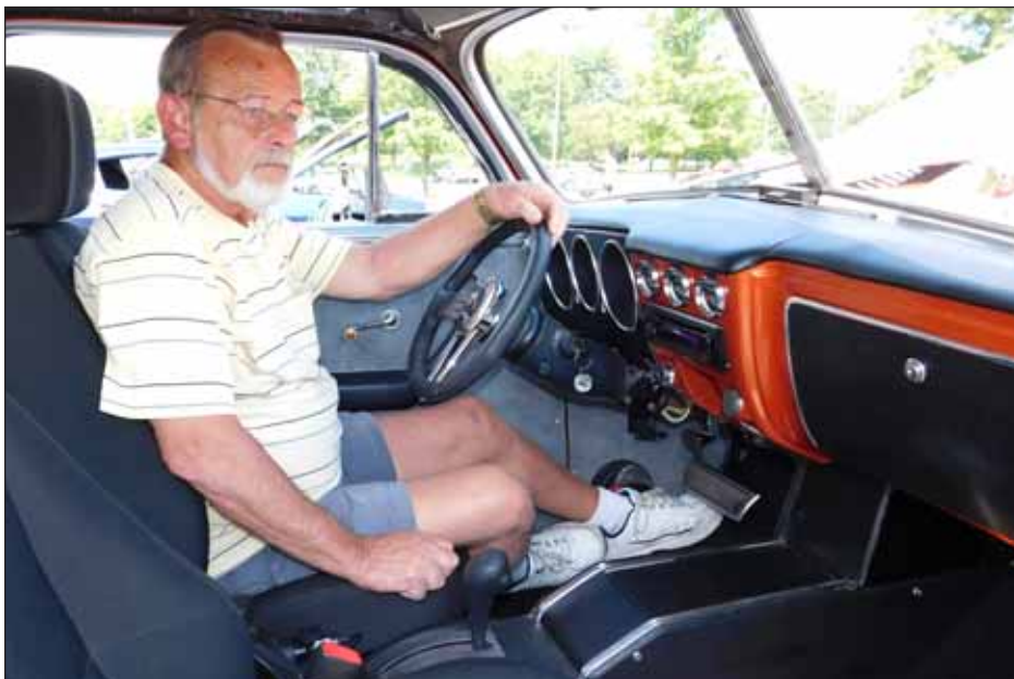
Dave Aker shows off the 13-year-old interior of his 79-year-old Pontiac. The oil pressure, temperature and charge gauges in that dash certainly aren’t stock, no more than the Kenwood stereo mounted below them. The dash itself was rescued from a 1968 Corvair, Aker said. Meanwhile, under the hood is a 326 engine from a 1965 Pontiac LeMans. And that decidedly 21st-century floor shifter came from a 2006 Pontiac Grand Prix.
